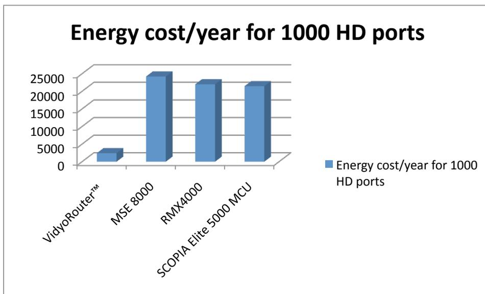
Depending on the product replaced by the VidyoRouter an annual energy cost savings of nearly an order of magnitude can be realized. The 10X advantage also continues in rack space and co-location costs as seen in the chart below. A standard rack provides 42U slots. Using the VidyoRouter, only 10 U slots would be required. Any of the transcoding based MCUs require almost 3 full racks to host the same number of ports.
