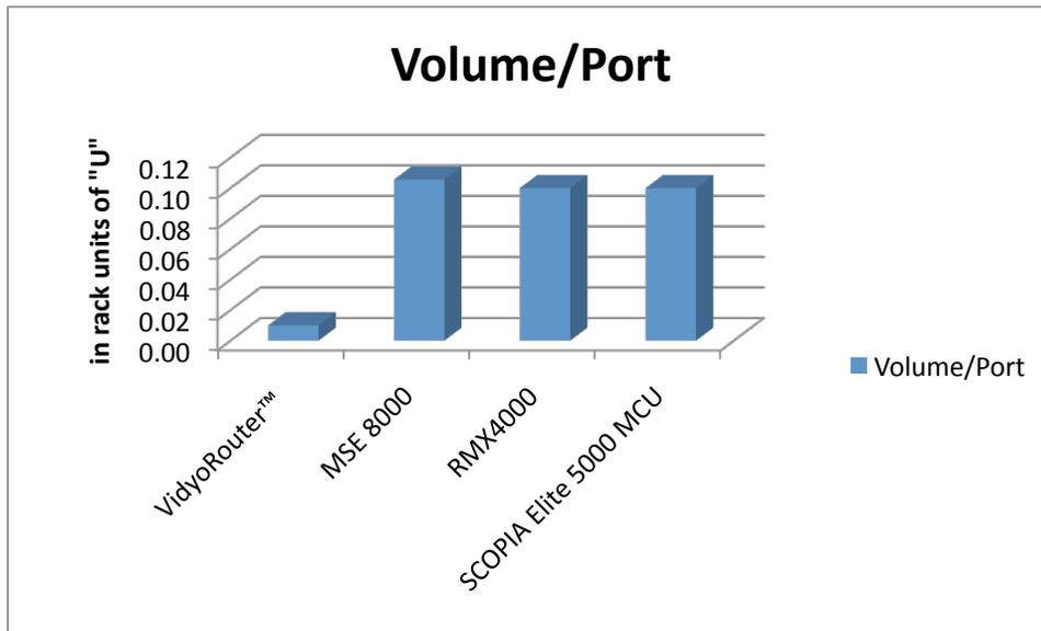
The charts clearly illustrate the simple fact that by eliminating transcoding functionality the VidyoRouter consumes far fewer resources to create a continuous presence display. The near factor of ten advantage in power consumption size and weight is consistent.
