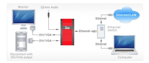
VGA2Ethernet is fully compatible with DirectShow in Windows, QuickTime in Mac OS X, and Video4Linux in Linux, meaning that it can be used in conjunction with any third party software that allows the use of an external camera as a video input. Alternatively, the VGA2Ethernet software, available as a free download, supports not only the viewing and saving of the DVI or VGA signal as an image or video, but also allows the user to:
