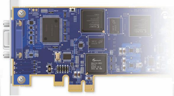
Epiphan Systems' VGA2PCle is an internal PCI express-based frame grabber designed for users that require high precision industrial VGA capture using an internal solution. The VGA2PCle can capture VGA streams at resolutions of up to 1920x1200 in a 24-bit palette, and is able to achieve a maximum capture rate of 80 frames per second.
