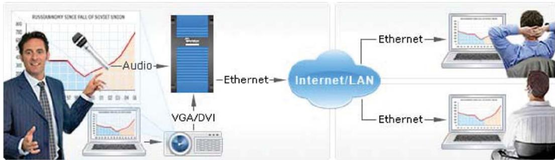
The VGA Broadcaster Lite is able to broadcast video in resolutions at up to 1600 x 1200 without any loss in quality or sharpness. The broadcasted video stream is then viewed with a media player such as QuickTime or VLC.
