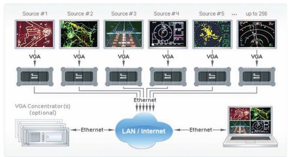
A VGA Grid device must be connected to the VGA output of each VGA source being monitored via a standard VGA cable. The VGA Grid devices are then connected to either a LAN or the Internet via a standard RJ45 Ethernet connector. Each VGA Grid device digitizes and compresses the analog VGA video signal and sends it over Ethernet to the VGA Bridge Gateway, which acts as a server and concentrator for up to 256 digitized VGA signals.
